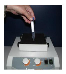
Several test tubes may be shaken at the same time, using the optional test tube adapters. These adapters are secured on the shaker table with wingbolts. Test tubes are plugged into "collets".
