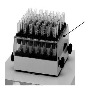
test tube adapter for 49 ea. dia. 12 test tubes, up to 80 mm long (P/N 549-82000-00) or test tube adapter for 36 ea. dia. 16 test tubes, up to 80 mm long (P/N 549-83000-00)
